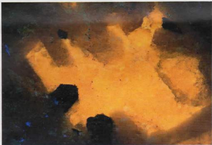
Fig. 2: Close-up of fluorescent sodalite. LWUV LED illumination, FOV approximately 4.0 mm, Travis A. Olds photograph. Although the fluorescent intensity of this Michigan sodalite is best described as moderate when illuminated by older-model Hg-vapor sources like the well-known portable 6-watt Mineralight® lamp, the fluorescence is quite brilliant in response to modern powerful multi-LED ultraviolet flashlights.
