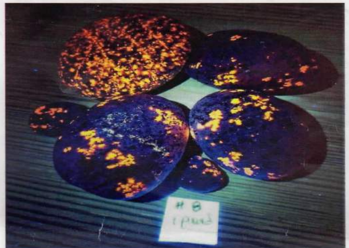
Fig. 1: A collection of "yooperlites" (syenite clasts containing fluorescent sodalite) collected from Lake Superior beaches in Chippewa and Luce counties, Upper Peninsula of Michigan. No dimensional scale but these specimens collectively weigh about one pound, as indicated on the paper note. LWUV LED illumination, Erik Rintamaki photograph.
